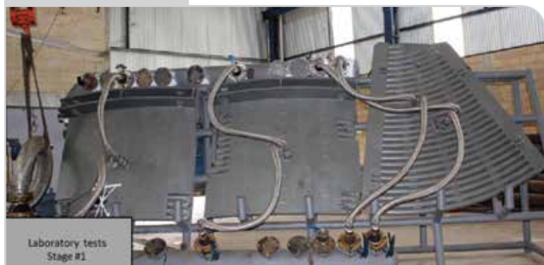
Panels mounted for conducting the laboratory tests of new leak detection technology.
