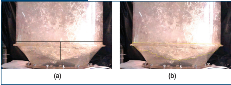
Jet penetration (a) and decarburization area (b).
