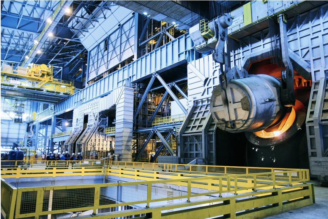
Figure 1: tkCSA converter (330 ton)
