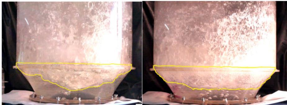
Figure 5: Comparison of Decarburisation area and Jet Penetration: (a) tkCSA 3-15 – DBL 400 mm and 120Nm<sup>3</sup>/h (b) tkCSA 3-13 - DBL 451 mm and 160Nm<sup>3</sup>/h.
