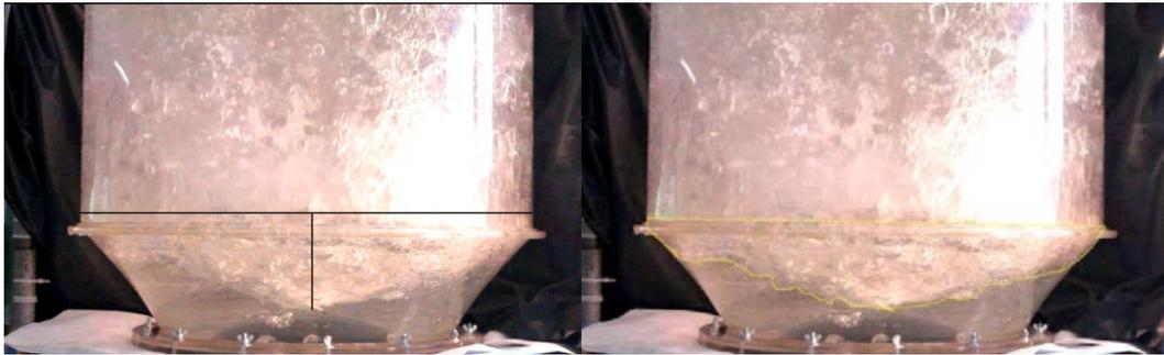
Figure 3: Jet Penetration (a) and Decarburisation Area (b)
