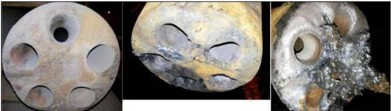
Fig. 18 - Nozzle wear and cartridge face due to differences between design conditions and operating conditions.
